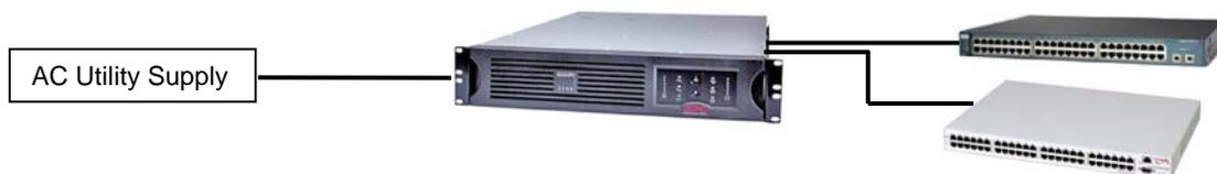
**Figure 3** provides an availability level of approximately five nines (99.999%) assuming a runtime of at least one hour. The utility supply feeds a UPS, such as an APC Symmetra RM<sup>®</sup> which in itself has a number of power modules configured to provide N+1 redundancy, which then supports the network switch with integrated PoE in the event of AC line disruption.
